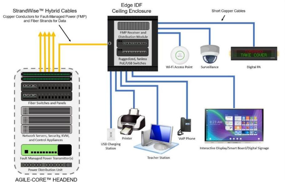
By distributing low-voltage DC power throughout a school, the AGILE-CORE system eliminates the bulk of AC-to-DC conversion required to power electronics. AC-to-DC conversion can result in significant power losses of up to 30 percent and introduce distortions into power distribution systems.
